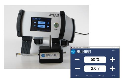
With the **vimpact-63**, structures can be excited precisely and reproducibly by setting the acceleration range of the hammer from 0 to 100 % in steps of 1%.
